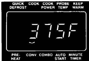
After the oven temperature has reached the temperature you selected, the oven beeps twice and the PREHEAT Indicator Light goes off. The set temperature will stay on the Display and the oven will hold that temperature up to 30 minutes, or until the food has been placed in the oven and START has been touched. **NOTE: The oven will automatically shut off and the Display will show the time of day if food has not been placed in the oven within 30 minutes.**
